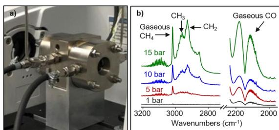
**Figure 2.** a) In house developed heatable, high pressure FTIR reaction cell. b) FTIR-spectra recorded after 60 min exposure of Fe<sub>3</sub>O<sub>4</sub> to the CO<sub>2</sub>/H<sub>2</sub>/He/Ne-feed (20/60/18/2; 50 ml/min) at different pressures.
