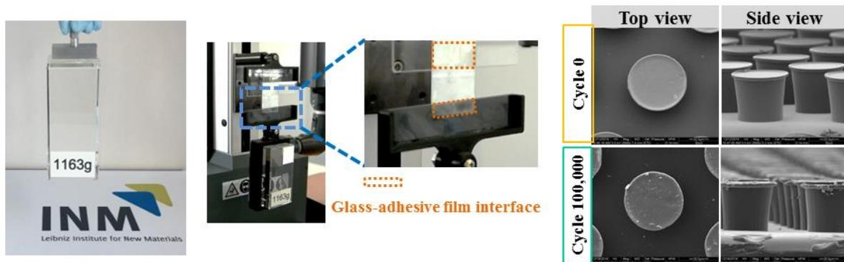
**Figure 3.** Photographs of handling a glass prism with mass 1.163 kg demonstrates normal adhesion (left) and shear adhesion (middle) of the adhesive film of U6L7-U6E4. Scanning electron images before and after 100,000 attachment-detachment cycles show good endurance of the adhesive film U6L7-U6E4 (right).
