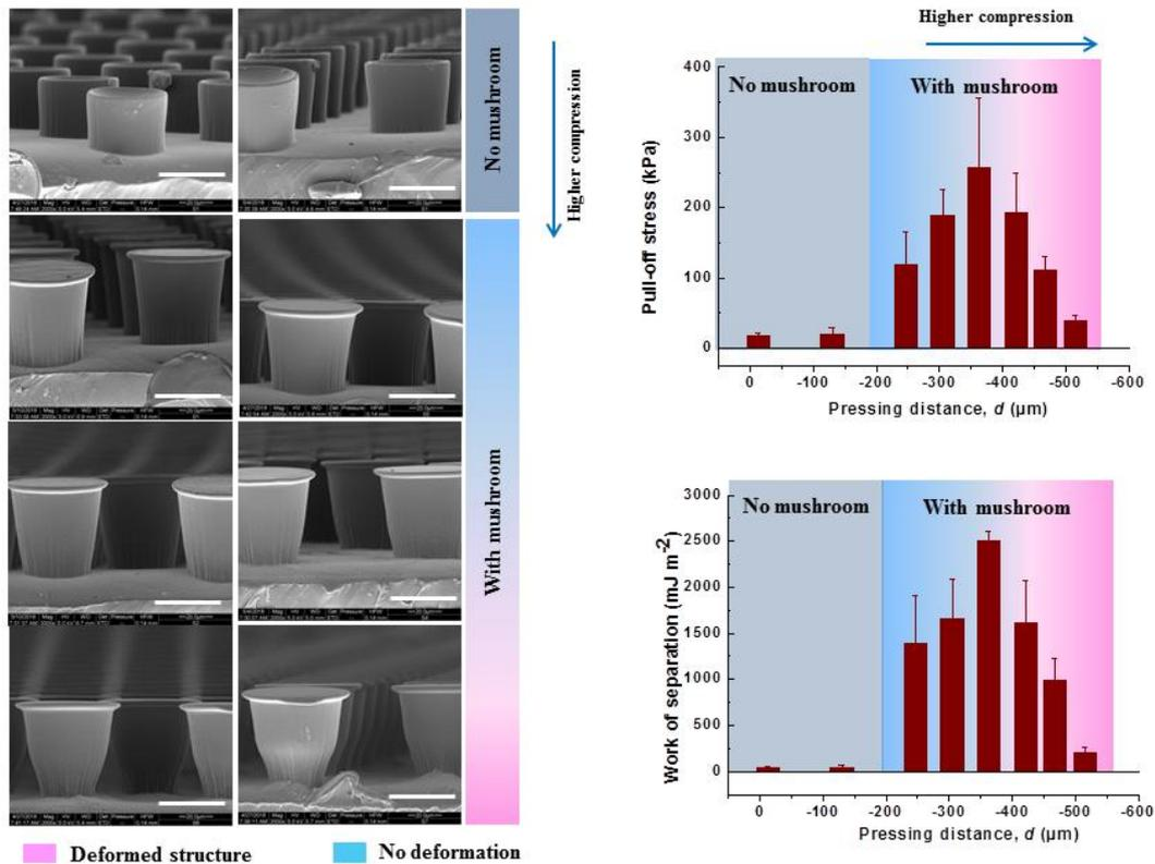
**Figure 1.** Scanning electron micrographs of UA16 micropillars fabricated with different compression (left). Scale bars are 40 µm. The dependence of pull-off stress and work of separation on compression (right).
