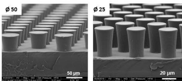
**Figure 2.** Scanning electron micrographs of the microstructures with pillar diameter of 50 µm and 25 µm.
